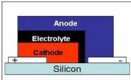
5) Deposit anode materials (note: the material proportions in these diagrams are NOT to scale).
