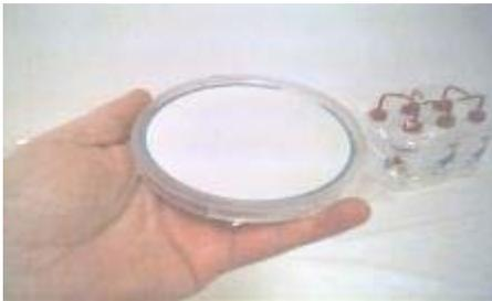
1) Start with a silicon wafer; this is a flat disc made of (you guessed it) silicon, which is commonly used in manufacturing integrated circuits.
