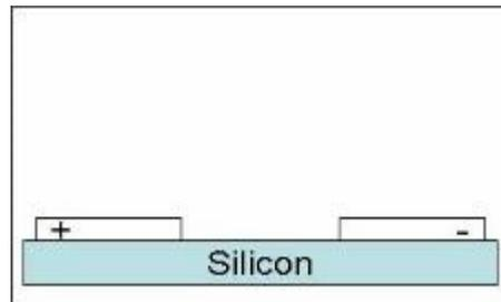
2) Add current collectors. These will serve as the connectors for the positive and negative poles of the battery.
