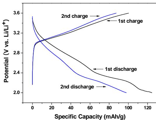
**Figure 3: Voltage profiles of the MnO<sub>2</sub> nanowires grown electrode for the first two cycles. The first**
