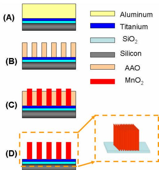
**Figure 1: Fabrication of a vertical array of MnO<sub>2</sub> nanowires grown on a SiO<sub>2</sub>/Si substrate:** (A) Deposition of 1 micron thick Al layer on SiO<sub>2</sub>/Si. (B) Anodization to fabricate an AAO consisting of a vertical array of cylindrical pores. (C) Growth of MnO<sub>2</sub> nanowires by electrodeposition. (D) Wet etching to realize the exposed vertical arrays of MnO<sub>2</sub> nanowires.
