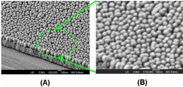
**Figure 2: FESEM micrographs of a vertical array of MnO<sub>2</sub> nanowires grown on a SiO<sub>2</sub>/Si substrate (A); zoomed image of a circled area in (A). A diameter of nanowires is about 80 nm.**
